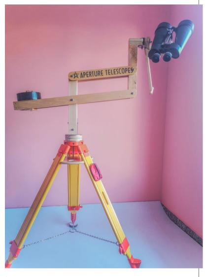
The height of the binocular eyepiece can be adjusted from 3.5 feet to 7.5 feet, keeping the same object in the field of view. Ideal when showing sky objects to large group of people. A sturdy wooden surveyor's tripod is included in the price. Wooden tripods and wooden mount is better at reducing vibrations. The binocular mount is constructed of the best marine plywood available, sealed and 4 layers of weather proof automotive PU spray, stainless steel and teflon.
